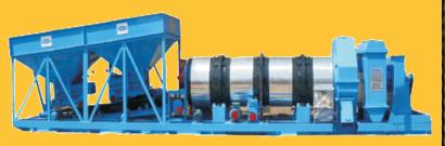
manufactured Asphalt Mix Plant reduces manufacturing costs and satisfies the changing industrial needs of the customers. The Asphalt Mix Plant has been manufactured for the mixing purpose of aggregates, sand and filler.
